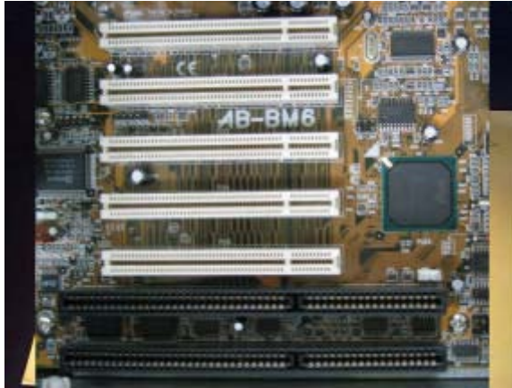
Figure 1.5 A motherboard of a PC with slots for PCI boards (five white connectors), and for ISA boards (two black connectors).
