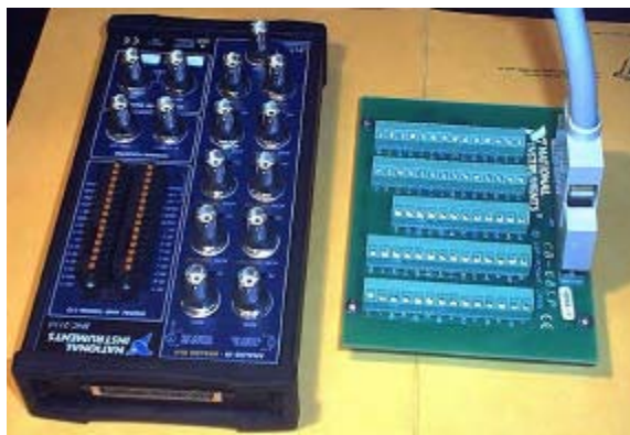
Figure 11.5 Two types of DAQ board connectors: (left) with terminals and BNC coax connectors, and (right) with screw terminals for unshielded cables.
