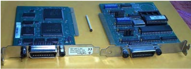
Figure 8.3 IEEE-4888 interface boards: for PCI bus (on the left) and for ISA bus (on the right).
