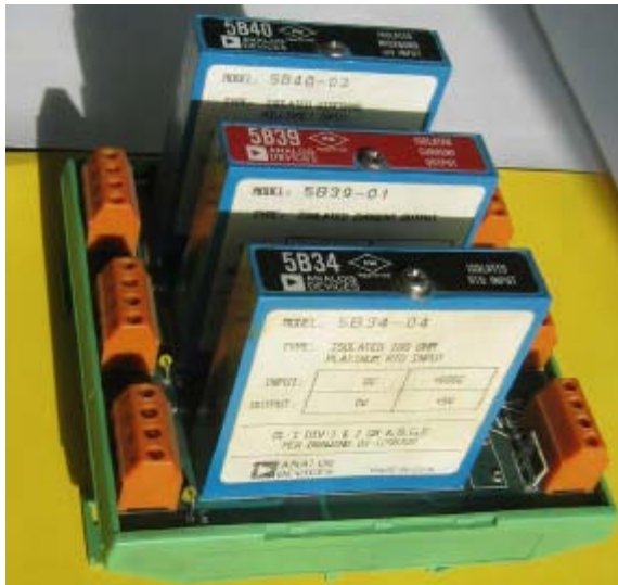
Figure 4.9 Three signal conditioners from the Analog Devices 5B series on an interface board (the 5B34-04 module for a Pt100 sensor is in front on the picture).
