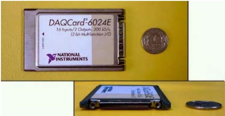
Figure 11.3 PCMCIA DAQ card: top view and side view of the I/O connector, next to a 1 Polish zloty coin for the comparison of dimensions.
