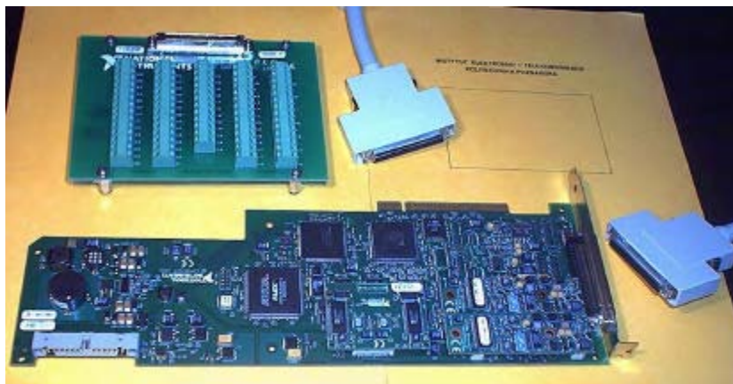
Figure 11.2 DAQ board for the PCI bus, with a connector and a cable.
